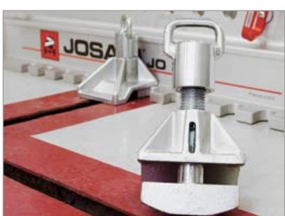
The JOSAM frame press is anchored to a frame rack in the floor.
