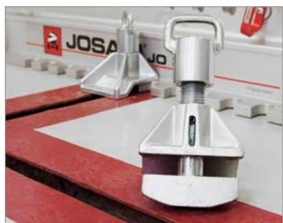
The JOSAM frame press is anchored to a frame rack in the floor.
