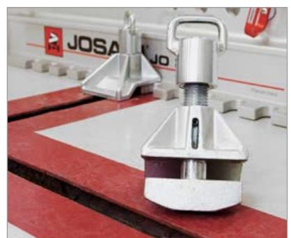
The JOSAM frame press is anchored to a frame rack in the floor.
