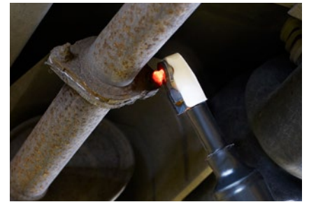
SERVICE APPLICATION REMOVE RUSTY EXHAUST BOLT
