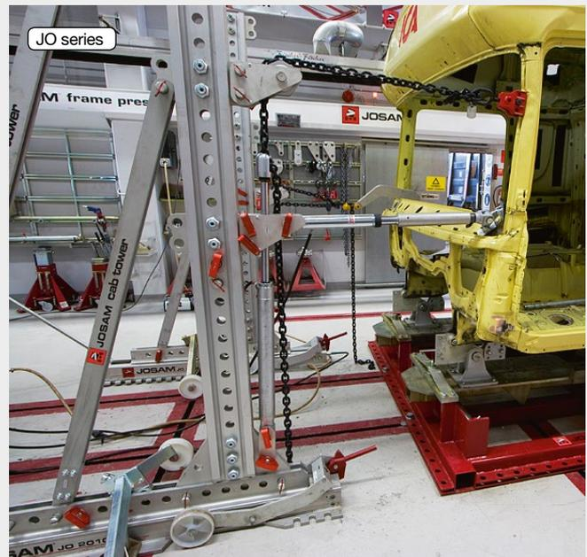
The I-beam system fixes the cab tower into floor beams which have been installed in the shape of a "cab square" or as a complete frame straightening bay.
