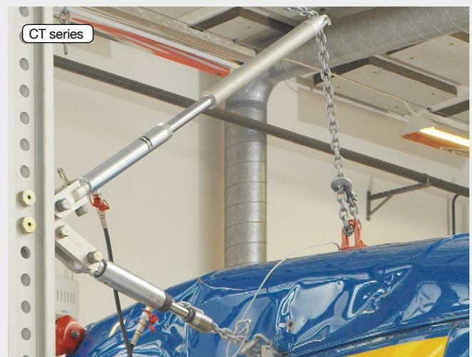
No matter which alternative is chosen, JOSAM cab tower can be utilized for many different repair jobs, thanks to its versatility. Here, for instance, a straightening job with advanced vector pulling is performed at 3-4 meters' height. In this case, our floor anchoring version is being used. Upwards vector pulling is only possible with this solution.
