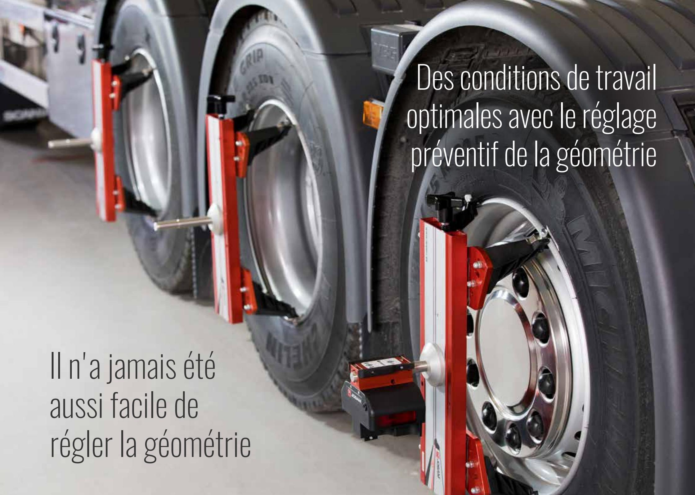
A close-up, perspective view of a truck's rear axle with three wheels. The wheels are mounted on silver hubcaps with multiple bolt holes. A red and white alignment machine is positioned around the wheels, with its arms and sensors in contact with the tires and hubcaps. The machine is used for adjusting the wheel geometry. The background is a blurred workshop floor.
