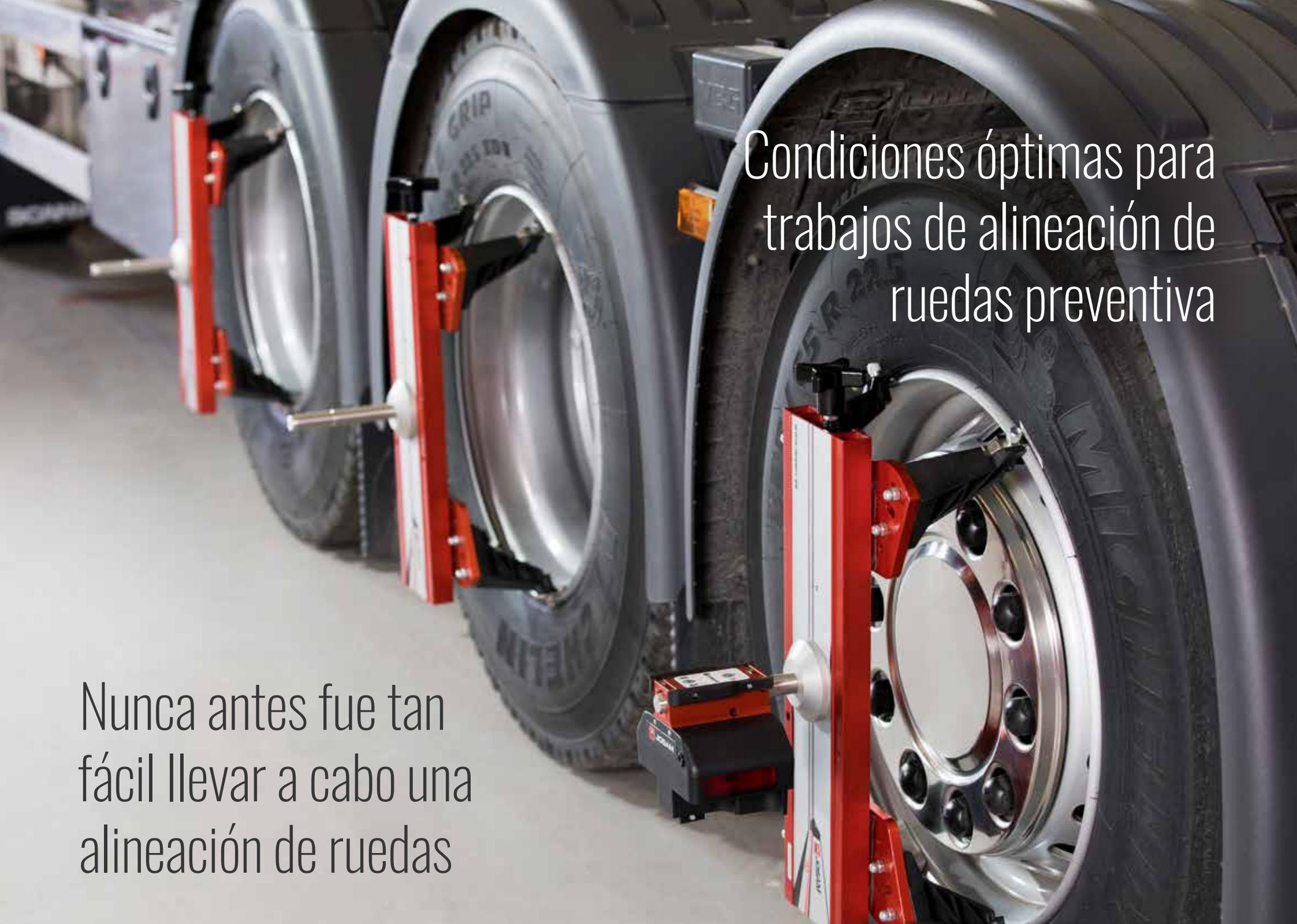
A close-up, perspective view of the rear three wheels of a truck. Each wheel is equipped with a red and white sensor assembly for wheel alignment. The sensors are mounted on the hub area of the wheels. The truck is on a light-colored floor, and the background is slightly blurred, focusing attention on the alignment equipment.
